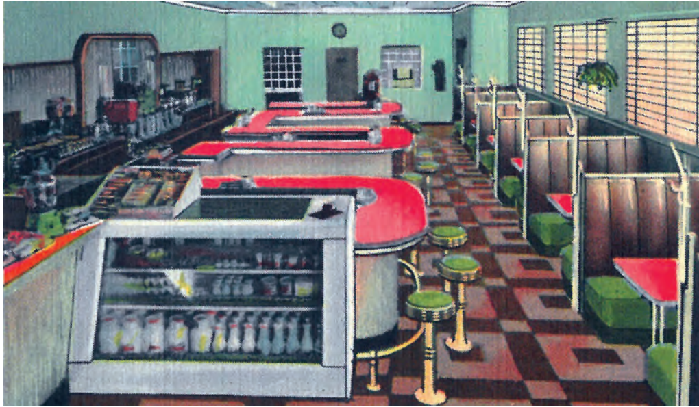
Figure 89. The layout of casual eateries varied but was generally organized around a lunch counter and kitchen galley that together made a U-shape, a highly efficient plan that minimized servers' movements.
